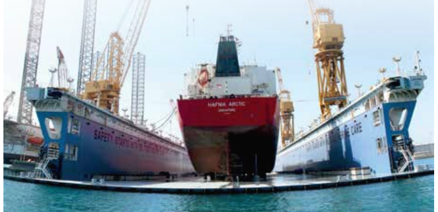
The product tanker Hafnia Arctic dry-docking for repair at N-KOM's newly developed floating dock, which is the largest of its kind in the world
