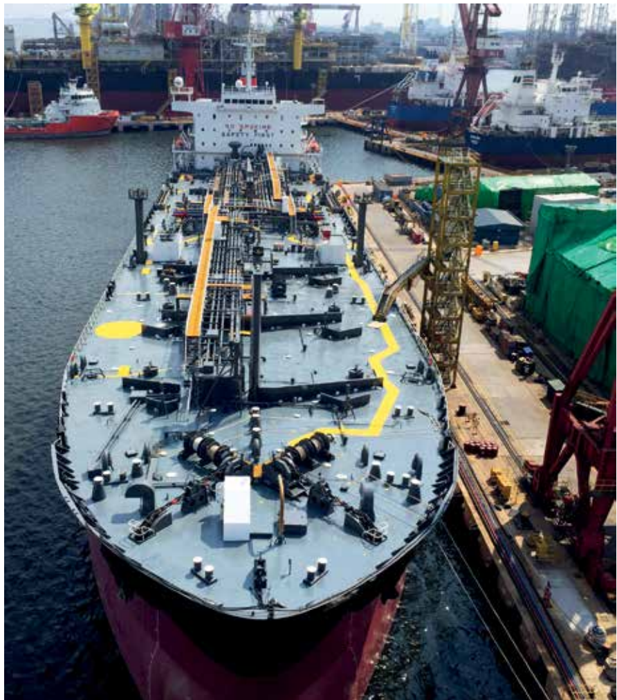
American Progress, an oil product tanker, underwent repair works such as hull painting and roller chock modification at Keppel Shipyard
